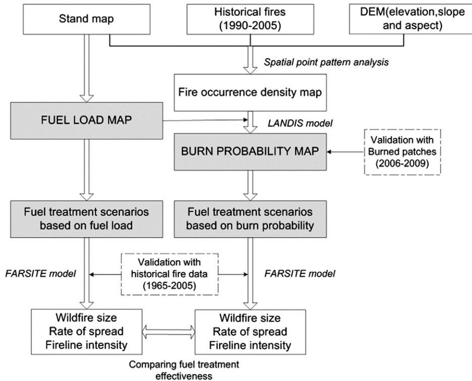
Fig. 2. The steps used to facilitate comparing the effectiveness of fuel reduction treatments based on burn probability vs. fuel load.
